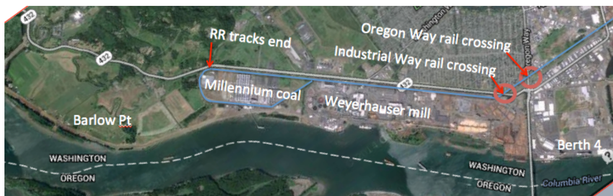
Figure 1: Map of the rail crossings and key properties related to SR 432. The blue line on the map above shows the “Reynolds Lead” section of the rail line: trains move from east to west off of the BNSF main line. The red circles depict the at-grade rail crossings at Oregon Way and Industrial Way that the $85M investment seeks to address.
