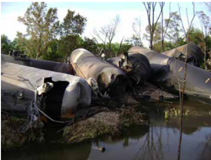
The May 2015 train derailment in Cherry Valley, IL, spilled about 324,000 gallons of ethanol, about 75 percent of the product carried in the 15 DOT-111 tank cars, from shell breaches, damaged top fittings, or damaged bottom outlet valves. Photo: NTSB
