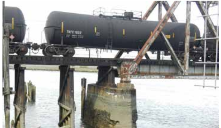
Oil tank cars with head shields, which are intended to decrease the chance of the cars breaking open during a derailment. Photo: Puget Soundkeeper
