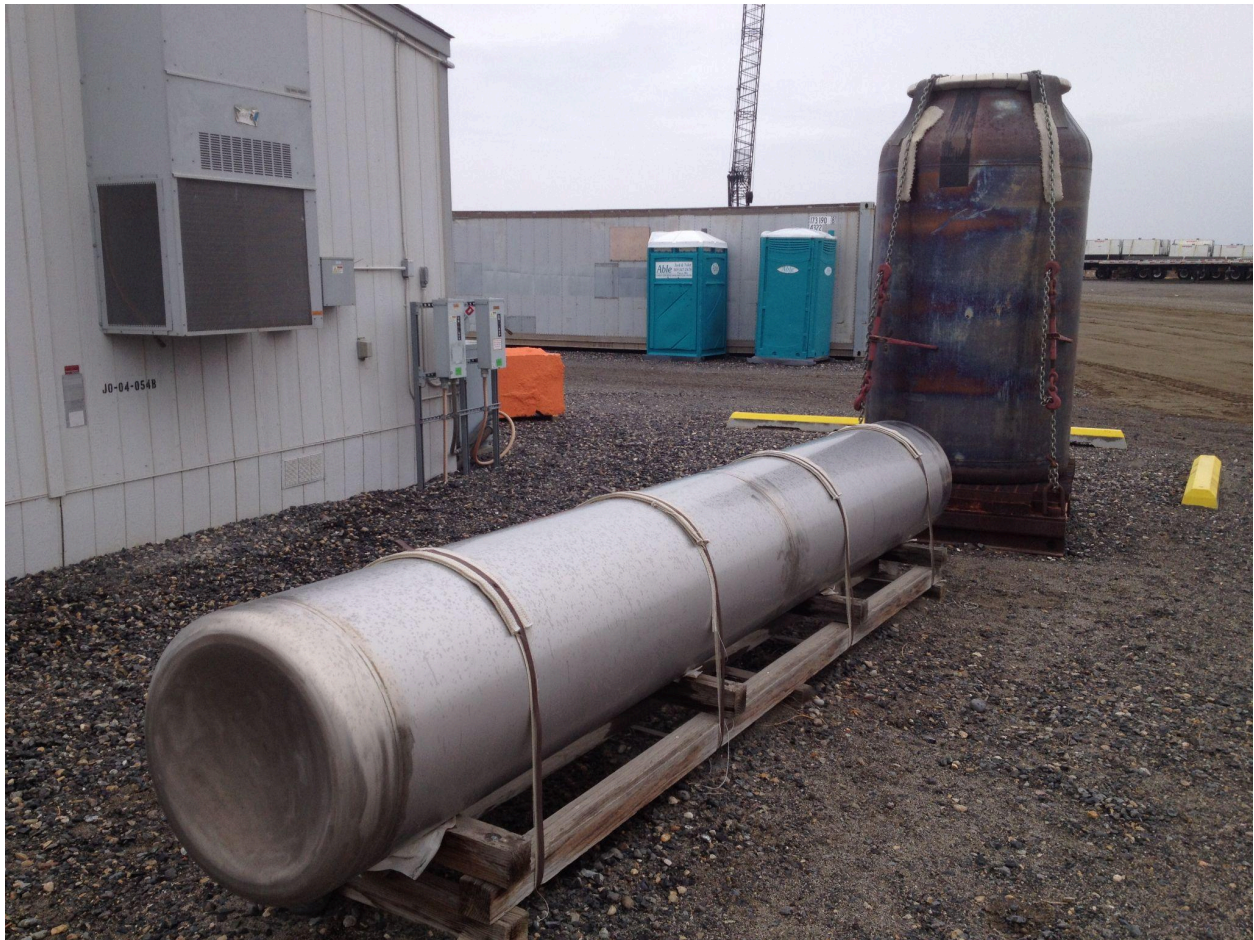
Above: The narrower canister would contain waste from the direct-feed HLW vitrification facility, and the wider canister would contain waste from the direct-feed LAW vitrification system. Photo by Columbia Riverkeeper. 2015.
